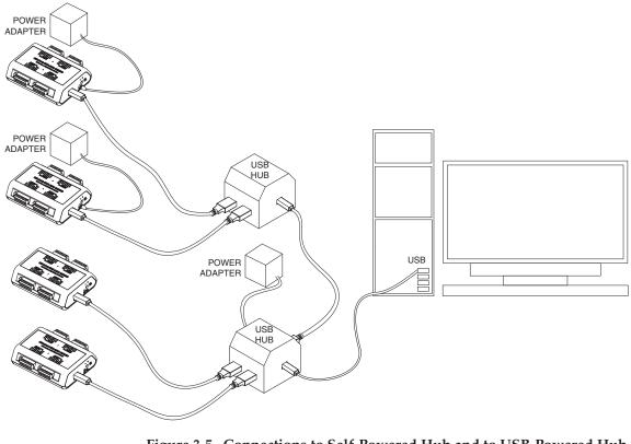
Figure 3-5. Connections to Self-Powered Hub and to USB-Powered Hub
